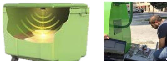
Figure 1. The placement of integrated sensor box inside the garbage containers
